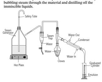
Safety tube (bottom of tube well below the level of water ... purpose: releases pressure, prevents explosions), steam trap (removes condensed steam), flask with whole cloves (more oil) and water, condenser, graduated cylinder (collect milky emulsion).
