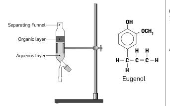
Anhydrous magnesium sulfate,  $MgSO_4$ , is added to the cyclohexane solution (organic layer) to remove any droplets of water. The hydrated magnesium sulfate and excess magnesium sulfate are removed by filtration. The organic solvent, cyclohexane (81°C), is then allowed to evaporate (water bath) leaving the pure oil behind.
