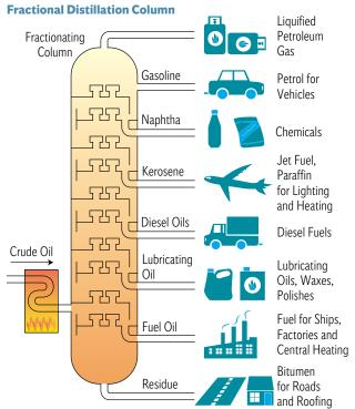
Fractional Distillation involves heating the crude oil and the different mixtures (fractions) are separated on the basis of their boiling points.
