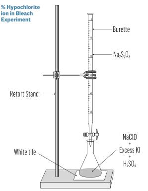
of the few drops of starch the solution in the titration flask goes blue-black (due to the presence of iodine). At the endpoint the solution goes colourless.
