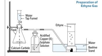
The water is added slowly from the tap funnel to allow for even evolution of ethyne gas. Three impurity gases ( $PH_3$ ,  $NH_3$ ,  $H_2S$ ) are also given off and these impurity gases are removed by bubbling all gases through acidified copper (II) sulphate solution. Ethyne gas is then collected by the displacement of water.
